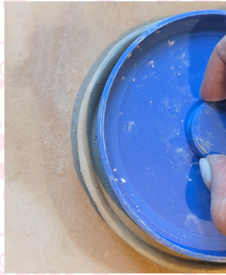
26. Give the mould a little twist & lift away from the clay
