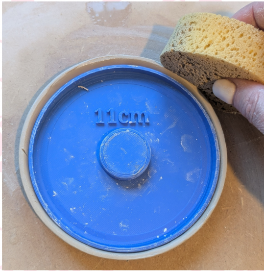
25. Very gently, smooth over the edges of your saucer with a damp sponge
