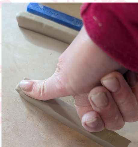
16. Here we've added an indentation on the end of the handle where it'll join with the mug by making a firm thumb print
