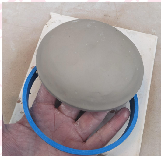
5. Press the mould and clay up through the cutter
